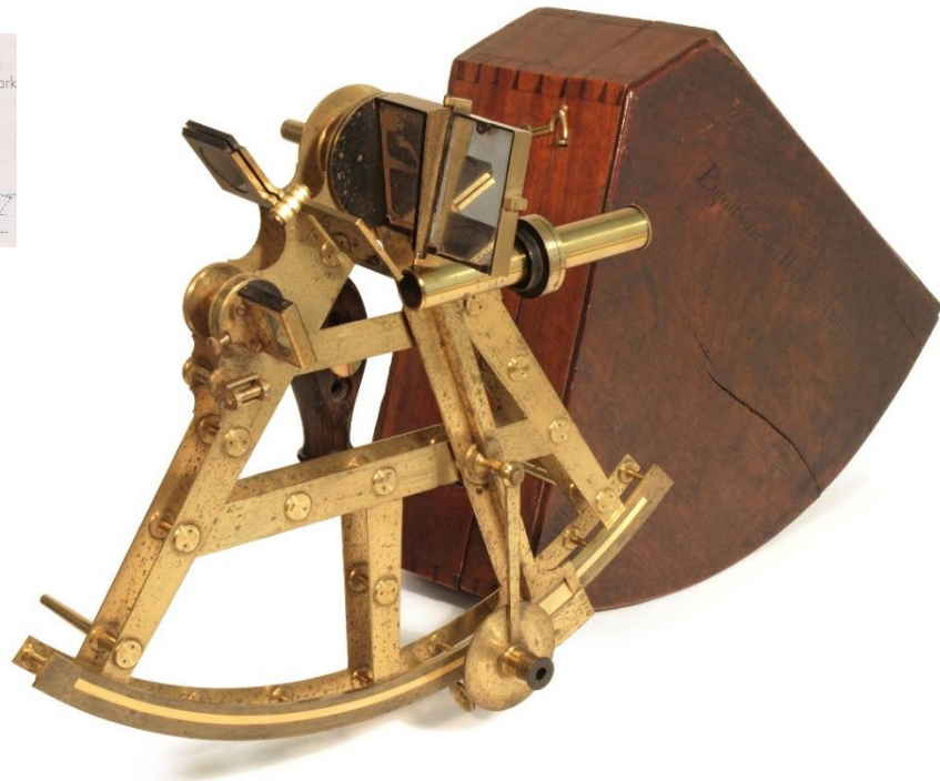
Fig. 4: Gauß's Vizeheliotrop (manufactured by Troughton, London, 1810). It was on the back of the 10 DM note. It was developed for a measurement campaign in the kingdom of Hanover, and its sensitivity allowed the study of the spherical excess of the curved earth's surface.
