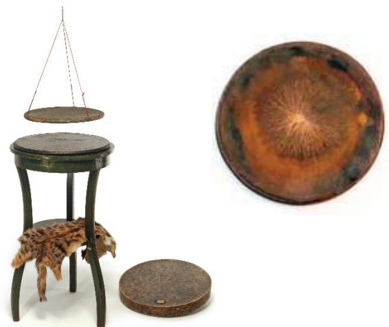
Fig. 3: Electrophorus and cat fur on the left at around 1780. With the tin foil coated wooden plate the charge could be separated and impressive electric sparks up could be generated. Lichtenberg figure for a positive charge on the right.
