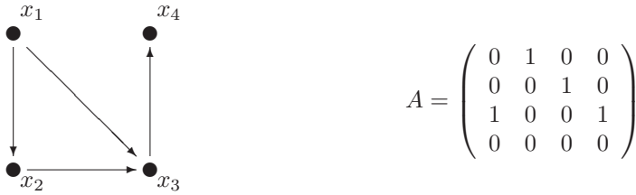
Figure 11.1: A directed acyclic graph containing and the corresponding adjacency matrix A .
